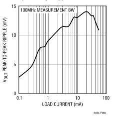
**Output Voltage Ripple vs Load Current**
