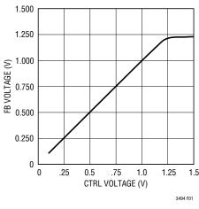
Figure 1. CTRL to FB Transfer Curve
