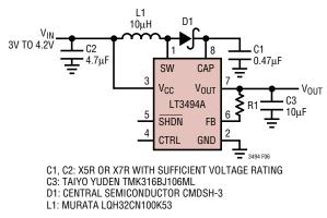
Figure 6. One Li-Ion Cell Input Boost Converter with the LT3494A
