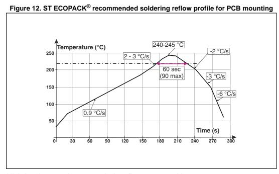
Note: Minimize air convection currents in the reflow oven to avoid component movement.
