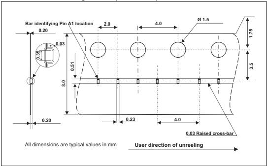
Figure 10. Tape and reel specification
